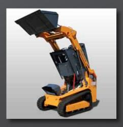
SERVICEABILITY A All-new cab support lock eliminates the need for a second person when raising the ROPS/FOPS structure for maintenance.
