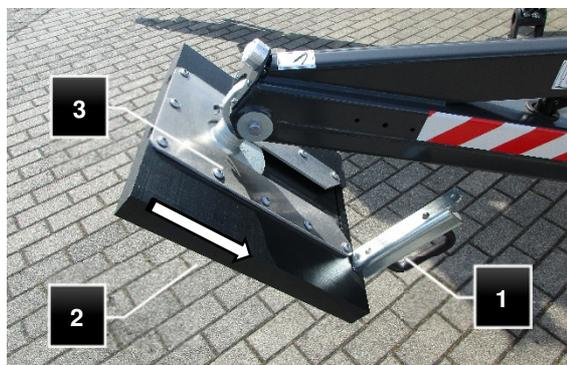
Fig.107 : Installer la plaque de support
